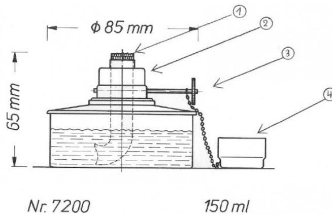
1. This burner is made of stainless steel. The burner has a volume of 150ml spirit. To fill the burner, you have to screw open the top (2), turn left to open, turn right to close.
